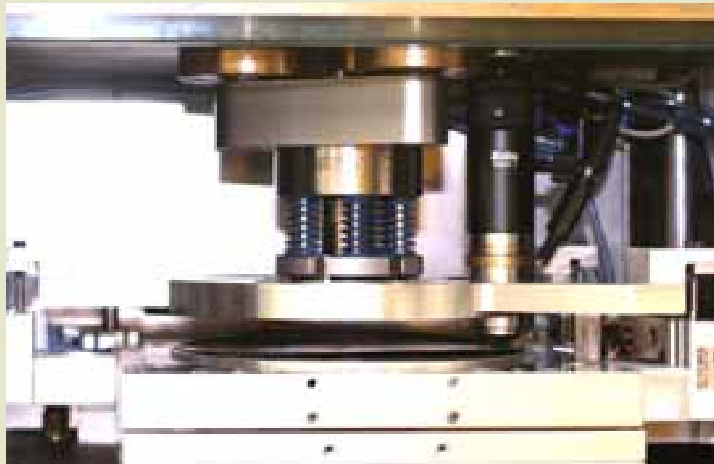
The P-145 uses high resolution optical technology and an Iterative Translation System
